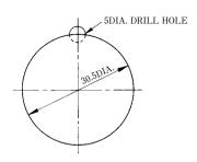
Note: The 5mm hole is used to stop whirl. If nameplates are not used or nameplate does not have any whirl-stop, the hole is not required.
