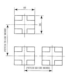
Refer to the dimensions specified below for proper mounting and separation from other magnetic materials. Units mounted closer together than specified may affect operations and result in unsatisfactory performance.
