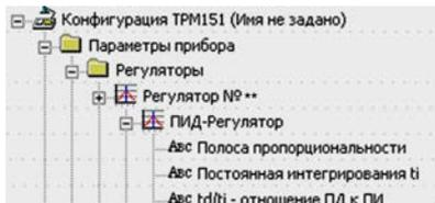
$$Y_i = \frac{1}{X_p} \cdot \left[ E_i + \tau_d \cdot \frac{\Delta E_i}{\Delta t_{изм}} + \frac{1}{\tau_{и}} \sum_{i=0}^n E_i \Delta t_{изм} \right]$$
